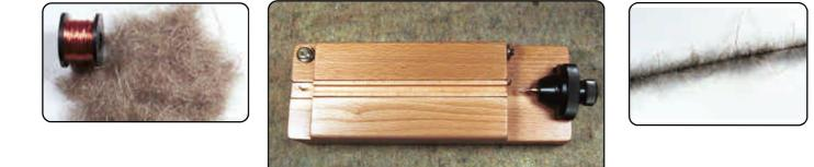
**NOTE:** There are two tension clips on the machine that need to be adjusted when changing wire thicknesses. This tension can be adjusted with a screwdriver and should be taught enough to firmly hold the wire when placed under the clip.
